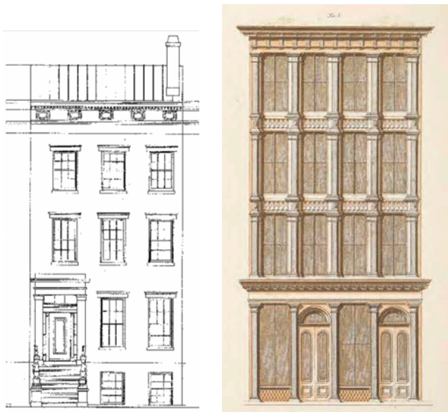
Fig. 10-11: A contemporary stone facade in the Greek Revival Style (l.) in comparison to a cast-iron facade by Daniel D. Badger's Architectural Iron Works (r.). The difference in the opening ratio is significant.
